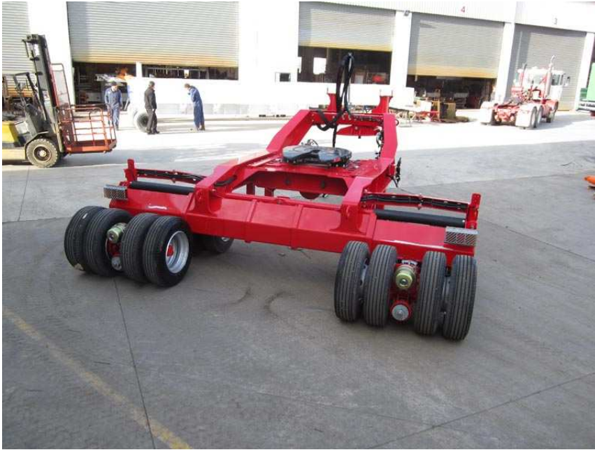
Figure A1. Widening dolly fitted with "rows of eight" axles shown in the widened position.
