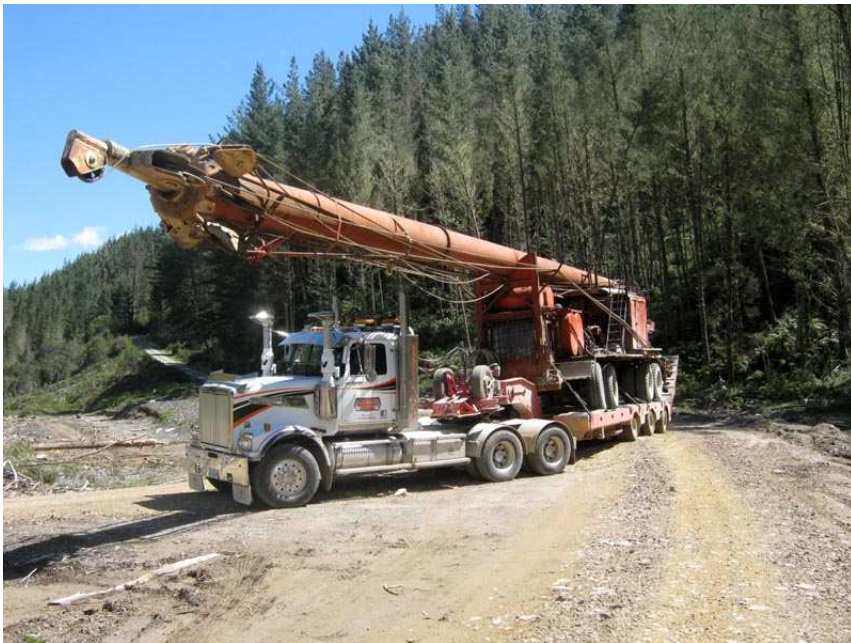
Figure A2. Log hauler being transported on a semi-trailer with three "rows of eight" axles.
