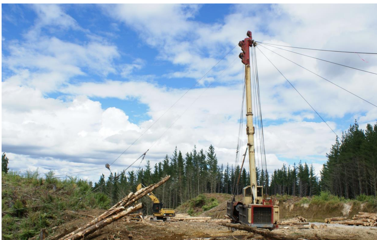
Pictured: A pole hauler at work in a cable logging operation.
