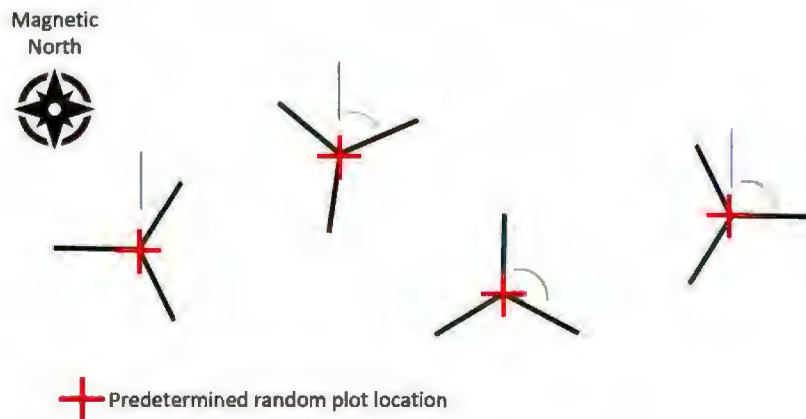
Figure 5: Sample orientation to a baseline to ensure sample remains unbiased to direction of accumulation of woody debris.
