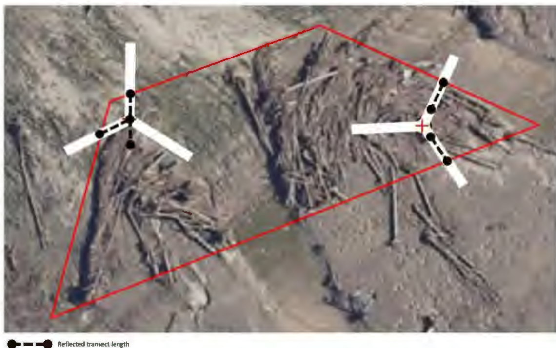
Figure 6: Edge plot mirage methodology for narrow debris piles or where transects fall into areas outside of the mapped debris extent.
