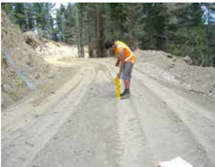
As part of his forest engineering studies a University of Canterbury student tests a forest road for strength/stiffness using a Clegg hammer
