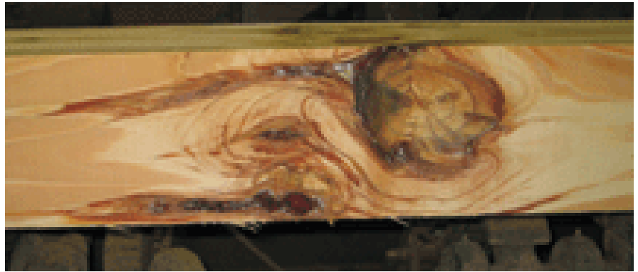
Central cant during saw ing show ing large infected branch w ith associated bark pockets.
