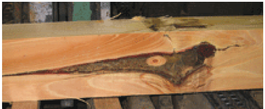
Large bark pocket associated w ith an infected whorl in the central cant of a pruned log .
