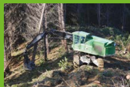
A remote buncher-feller does the job with the nearest human 100m away.
