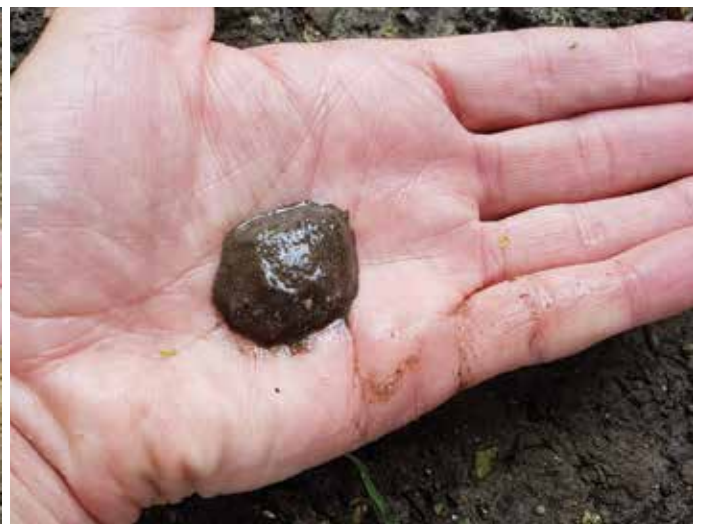
Left: The process of rolling a worm is a simple test for clay content. Right: The pat and tap test for silt
