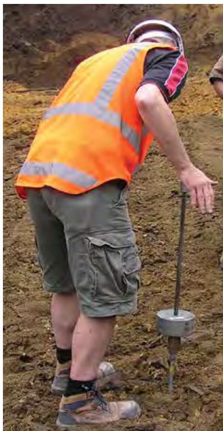
Above: A cone penetrometer being used. Right: The chart showing the number of blows to reach a given depth, overlaid with the estimated CBR value
